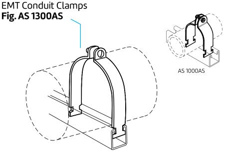
For EMT, IMC, GC, Pipe, or O.D. Tube
